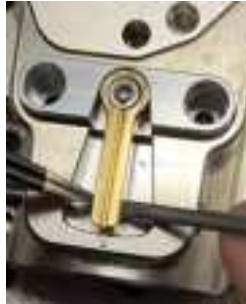
Figure 4.1: Removing the intracavity filter assembly.
