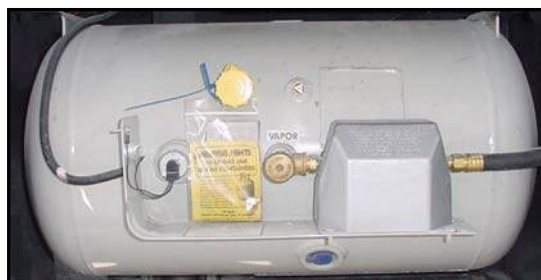
Figure 2-5. Liquid Propane Tank
