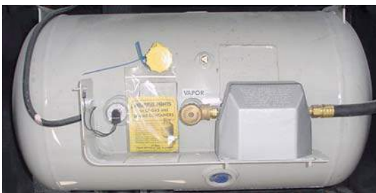
Figure 3-6. Liquid Propane Tank
