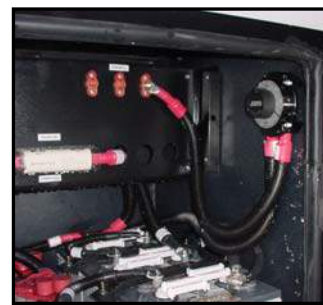
Figure 7-8. Rotary Switch to Disconnect “House” Batteries
