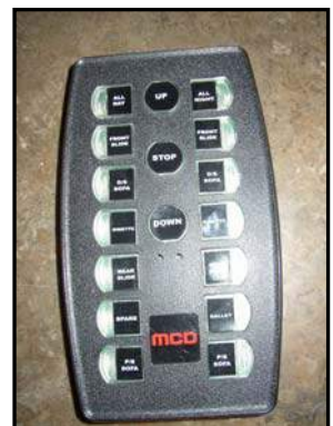
Figure 10-4. Control for Living Area Power Shades
