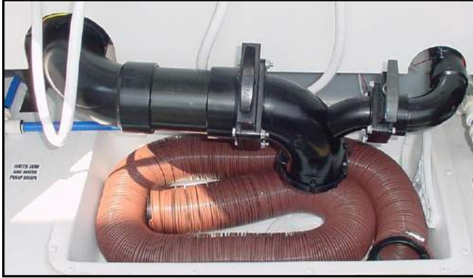
Figure 11-14. Sewer Hose and Drain Connections
