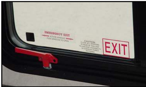
Figure 13-2. Emergency Exit Window
