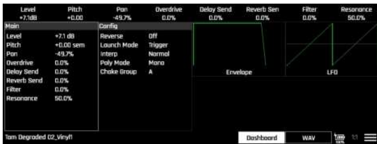
Figure: One-shot track dashboard showing common voice parameters
