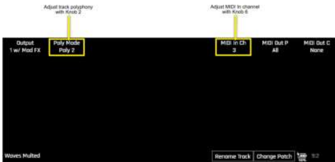
Track Configuration screen showing MIDI In Ch parameter setting
