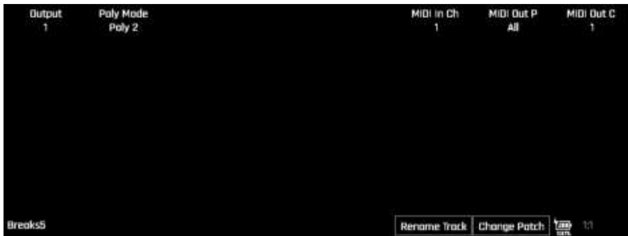
Figure: Slicer Track Config with MIDI In Channel 1
