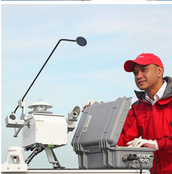
Figure 6 Pyrheliometers mounted on solar trackers.
