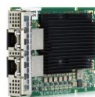
Ethernet 10Gb 2-port BASE-T OCP3 Adapter
