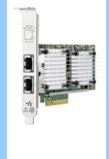
Ethernet 10Gb 2-port BASE-T Adapter
