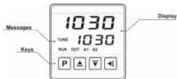
Fig. 02 - Identification of the parts referring to the front panel
