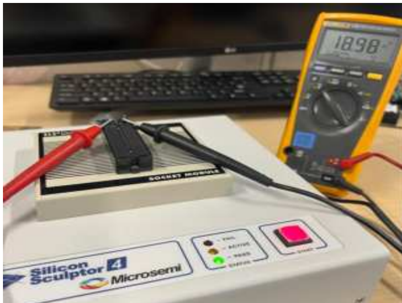
Figure 1-9. Measuring the Voltage of Pin 1
