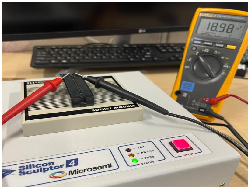
Figure 1-9. Measuring the Voltage of Pin 1
