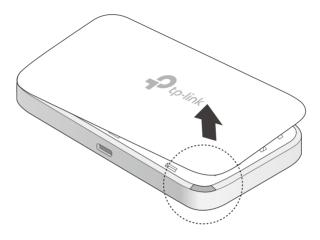
2. Slide and lift up the SIM card slot cover and insert the SIM card. And then slide to lock the SIM card slot.
