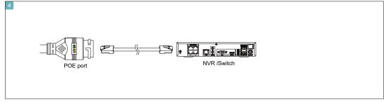
All external devices should be powered separately. There is no power voltage from the camera.
