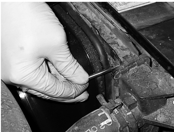
Install temp. probe near inlet hose...
