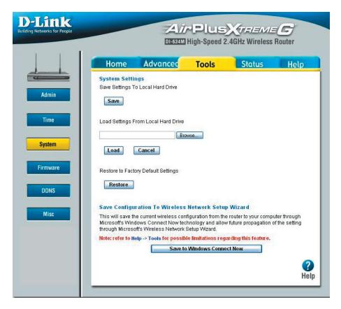
The current system settings can be saved as a file onto the local hard drive. The saved file or any other saved setting file can be loaded back on the Broadband Router. To reload a system settings file, click on **Browse** to browse the local hard drive and locate the system file to be used. You may also reset the Broadband Router back to factory settings by clicking on **Restore**.
