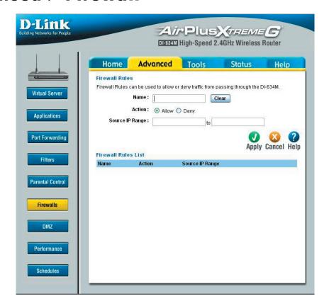
Firewall Rules is an advanced feature used to deny or allow traffic from passing through the DI-634M. It works in the same way as IP Filters with additional settings. You can create more detailed access rules for the DI-634M. Firewall Rules contain all network firewall rules pertaining to IP (Internet Protocol).
