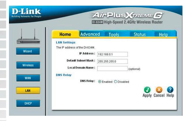
LAN is short for Local Area Network. This is considered your internal network. These are the IP settings of the LAN interface for the DI-634M. These settings may be referred to as Private settings. You may change the LAN IP address if needed. The LAN IP address is private to your internal network and cannot be seen on the Internet.
