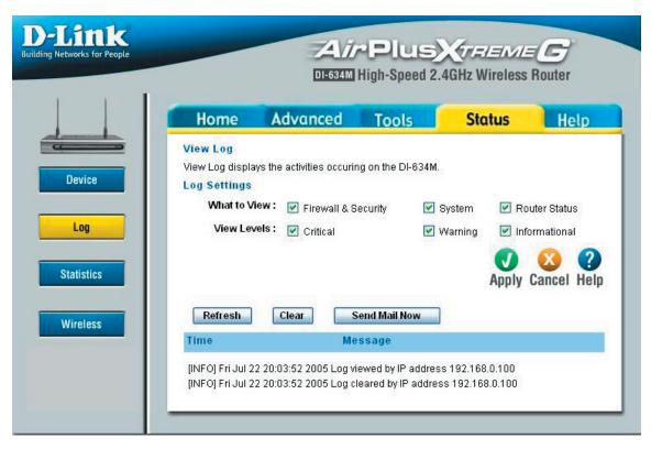
The Broadband Router keeps a running log of events and activities occurring on the Router. If the device is rebooted, the logs are automatically cleared. You may save the log files under Log Settings.
