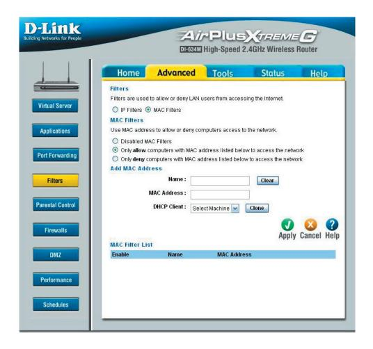
Use MAC (Media Access Control) Filters to allow or deny LAN (Local Area Network) computers by their MAC addresses from accessing the Network. You can either manually add a MAC address or select the MAC address from the list of clients that are currently connected to the Broadband Router.
