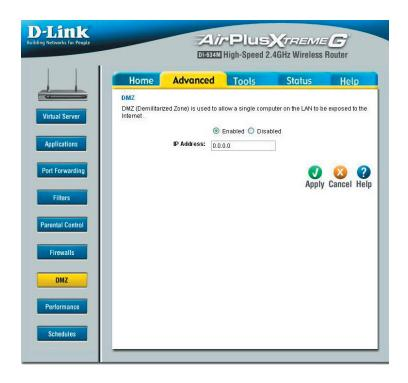
If you have a client PC that cannot run Internet applications properly from behind the DI-634M, then you can set the client up for unrestricted Internet access. It allows a computer to be exposed to the Internet. This feature is useful for gaming purposes. Enter the IP address of the internal computer that will be the DMZ host. Adding a client to the DMZ (Demilitarized Zone) may expose your local network to a variety of security risks, so only use this option as a last resort.
