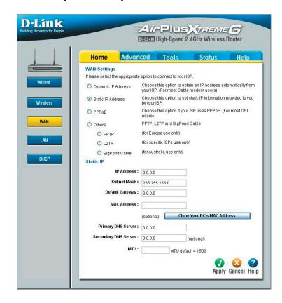
Choose Static IP Address if all WAN IP information is provided to you by your ISP. You will need to enter in the IP address, subnet mask, gateway address, and DNS address(es) provided to you by your ISP. Each IP address entered in the fields must be in the appropriate IP form, which are four octets separated by a dot (x.x.x.x). The Router will not accept the IP address if it is not in this format.
