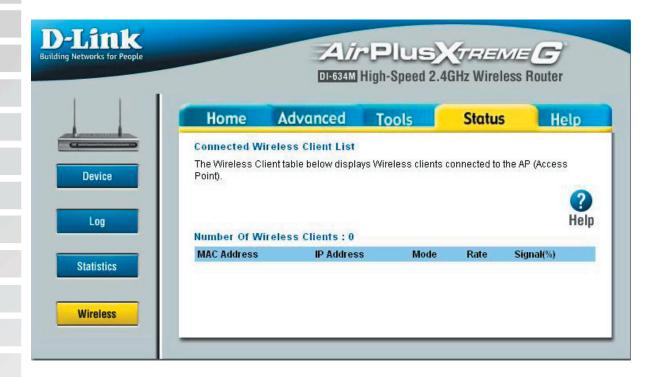
This screen will display any wireless client that is currently connected to the wireless router. The connected time and MAC address will be displayed.
