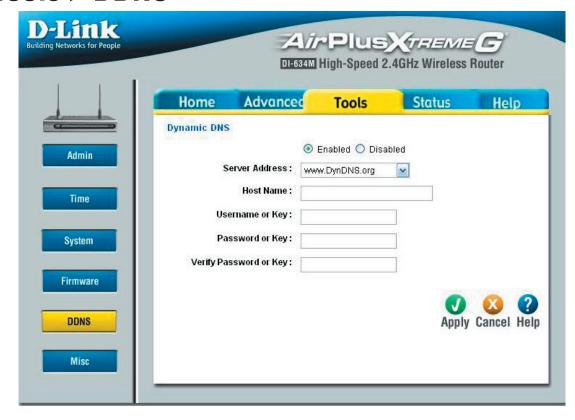
**DDNS:** If **Enabled**, this will allow you to use the DDNS update client built into the router.
