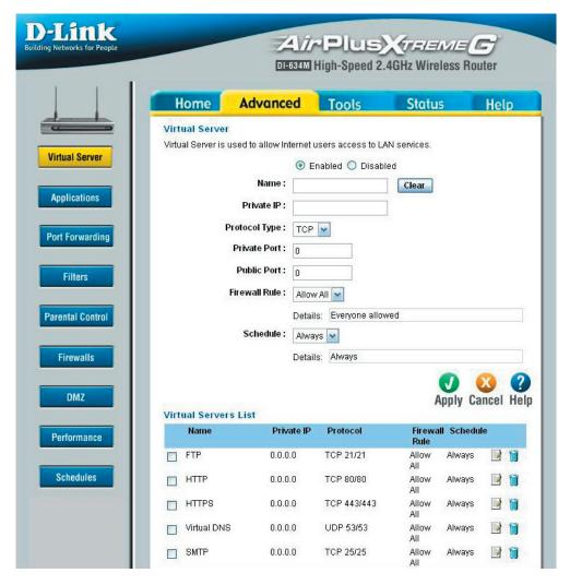
The DI-634M can be configured as a virtual server so that remote users accessing Web or FTP services (for example) via the public IP address can be automatically redirected to local servers in the LAN (Local Area Network).
