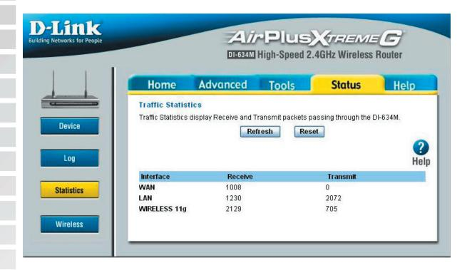
The screen above displays the Traffic Statistics. Here you can view the amount of packets that pass through the DI-634M on both the WAN and the LAN ports. The traffic counter will reset if the device is rebooted.
