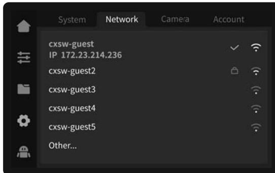
① Check the machine IP on the machine screen: Settings → Network.
