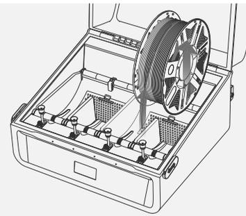
Unloading filament: First, make sure that the filament is not in the extruder, in this case, just pick up the filament and pull it out; if it is in the extruder, click the Retract button first, wait for the filament to return to the CFS, and then take out the filament.
