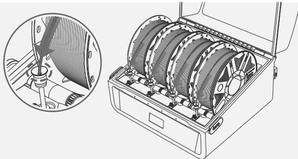
Loading filament: Put the filament into the CFS, align the filament head with the Teflon tube of corresponding silo, push it in gently, and let go after feeling the pulling force. The filament will be automatically loaded.
