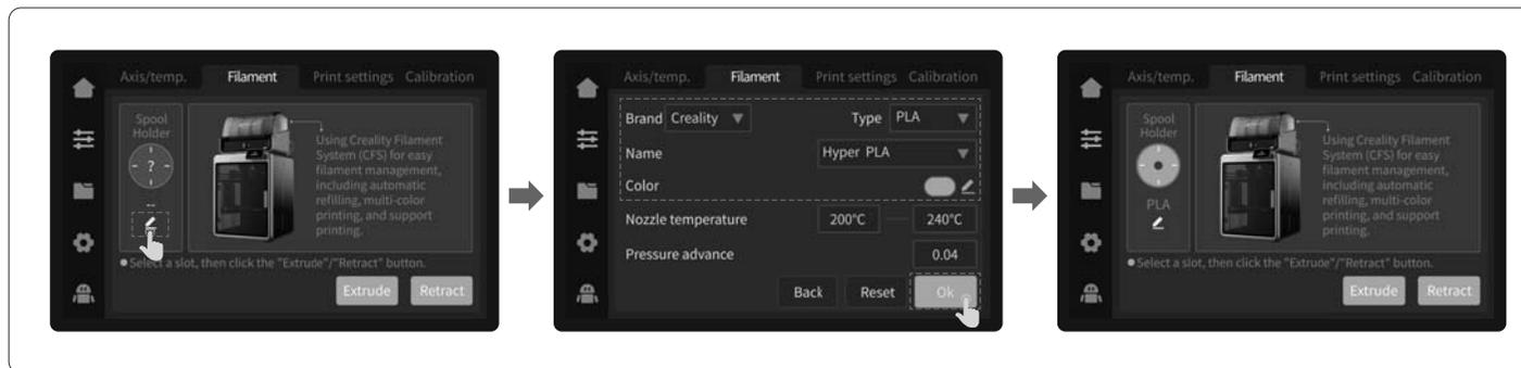
3 Manually tap the screen to set the filament information: Adjustment page → Filament → Edit (as shown below the material rack). Set the filament brand, type, name, and color, and finally click "ok" to save the settings.
