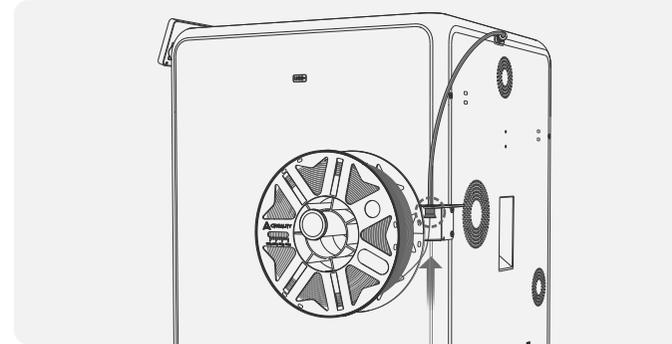
2 Thread the filaments into the Teflon tube and push gently until they cannot be pushed.
