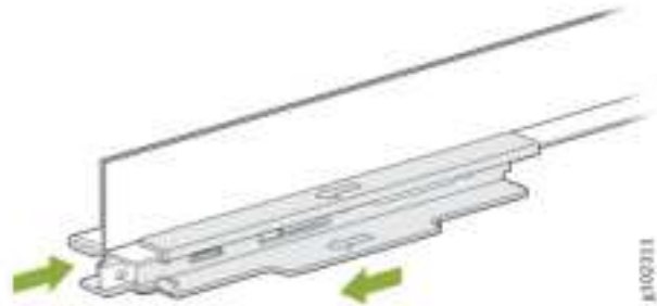
Figure 15: Attach the ADPR-ADP-RT15 Adapter to the T-Bar
