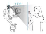
The tracking module only supports following people and prioritizes those close to the lens and near the center of the view. The subject tracked should be 1 m to 3 m away from the tracking lens.
