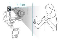
**Stop tracking:** Show the **gesture** or press the trigger again. The indicator turns solid red.
