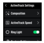
If no intelligent tracking module is connected, No Signal Input will display on the screen. When the intelligent tracking module is connected, composition, ActiveTrack Speed and gestures can be set on this page.
