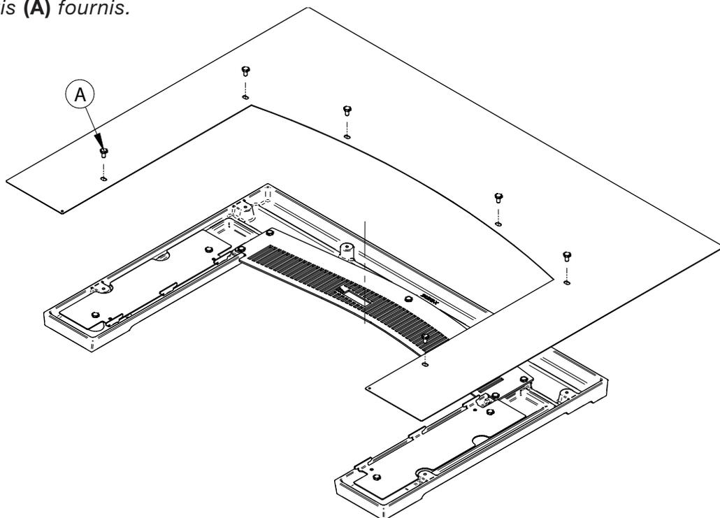
3. Align the faceplate hooks with the insert and slide the faceplate down to hook it on the insert.
