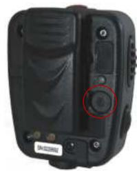
1. Ensure your **Elite™** speaker-microphone (SM) is charged before use. Before plugging your SM into the Android device, set the configuration to **5** by pressing the rear button for 4 seconds. The SM will then beep twice in quick succession.
