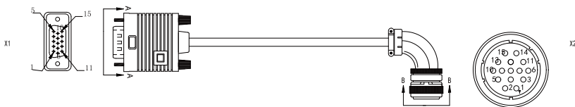
Cable for resolver encoder used by flange 200/263 motor
