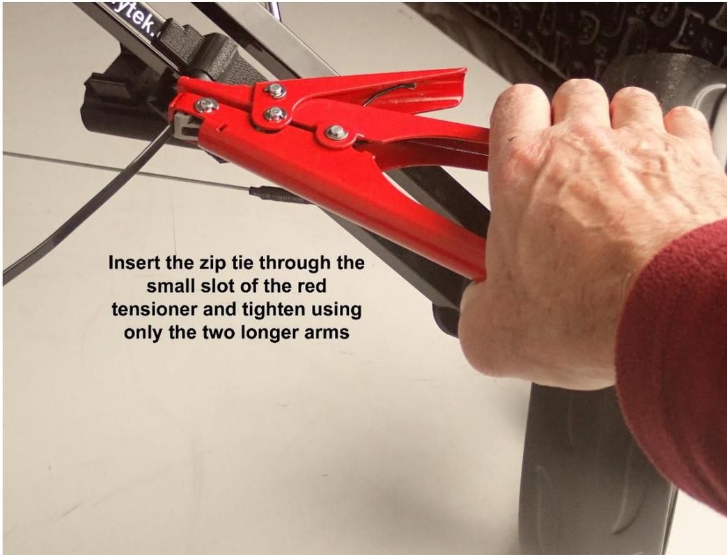
**Insert the zip tie through the small slot of the red tensioner and tighten using only the two longer arms**
