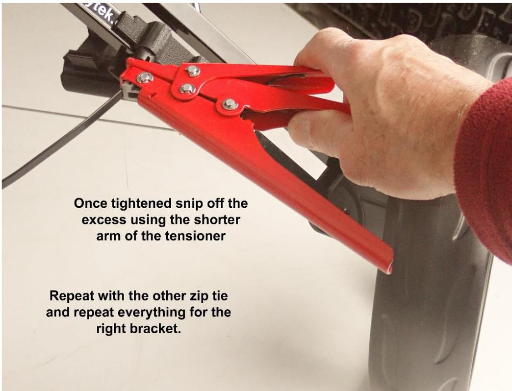
**Once tightened snip off the excess using the shorter arm of the tensioner**
