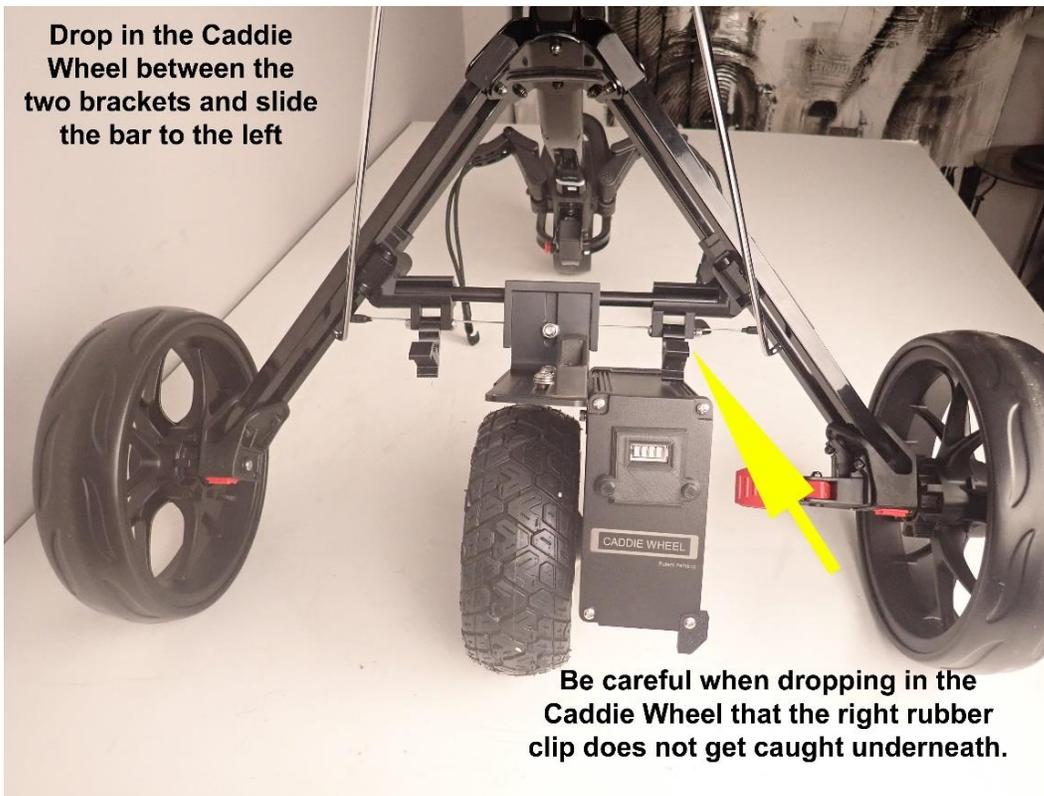
To lock the press firmly on the lower arm of the rubber clip. Make sure that it is firmly locked in. You should hear two clicks
