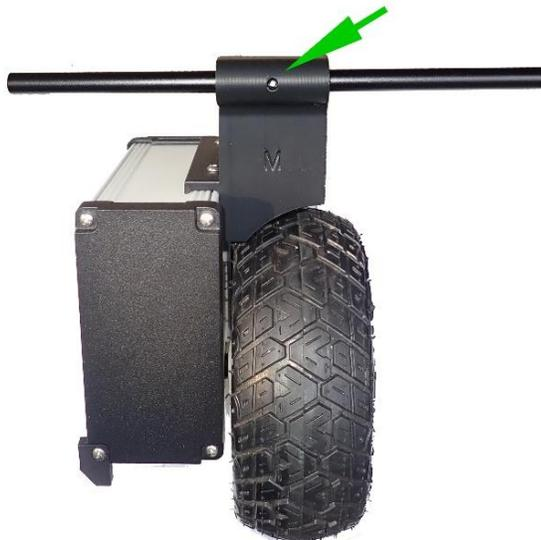
**Thread in the screw and tighten using the allen key**
