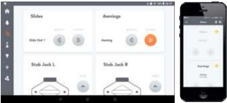
Figure 11: Motors Screen. Only one motor may be operated at a time and motor operation on other devices will be disabled.
