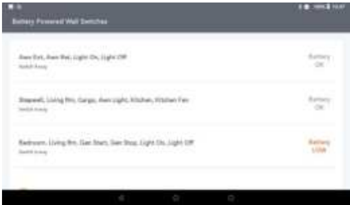
Figure 20: Battery Powered Wall Switches Settings. LOW indicates that the battery in the wall switch needs replacing..
