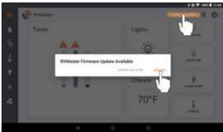
Figure 19: Click on the “Update Available” notification, then press “Update” at the prompt to update the firmware on the RVMasterNode .
