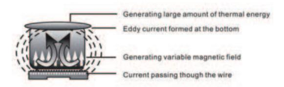
The Induction Cooker is mainly based in the electromagnetic induction technology. The sophisticated electronic circuitry of the induction hob produce high frequency electromagnetic field resulting high heat energy which heats up the bottom of the vessel and pass on the food directly effecting very fast cooking with thermal efficiency up to 93%.
