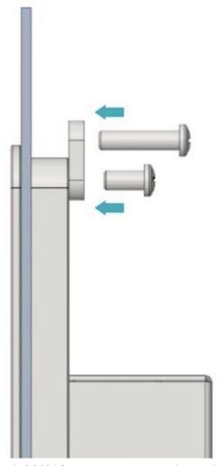
5. Use 4xM4\*10 screws to pass through the buckle and tighten it clockwise to fix the buckle to the device; then use 4xM4\*16 screws to pass through the screw hole (threaded hole) of the buckle and tighten clockwise to the end through the buckles.
