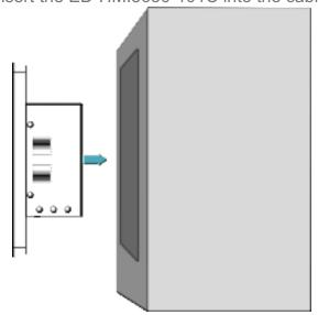
4. Align the screw hole (unthreaded hole) of the buckle with the buckle installation hole on the device.
