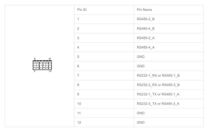
The pin names of the RS485 port corresponding to CM5 are as follows:
