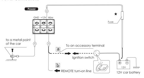
\* Place the fuse in the power supply lead as close as possible to the car battery.
