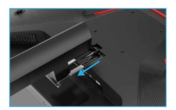
Hold down the "PUSH" button and exit the column assembly according to the operation direction in the figure;
