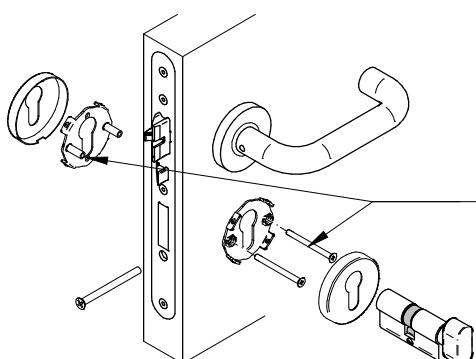
(Eng) It is advisable to mount the keyhole roses using a system composed of screws and bolts. By screwing the inner part to the outer part with through screws, you can achieve a higher level of security. However, if you use lag bolts for the installation, these must be long enough to fasten the plate without touching the mortise lock.
