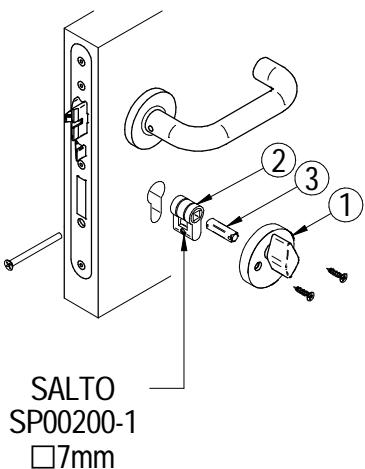
The diameter of the rose must be at least 54mm to cover the door hole. To use ① thumbturn with the SALTO lock, you need to use cylinder adapter ②. To do this, the square spindle ③ must be 7mm.
