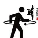
Y-axis calibration, aircraft vertical rotation
