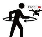
X-axis calibration, aircraft horizontal rotation
