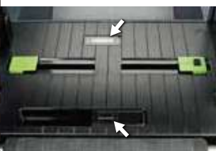
Twin-Eyed sensor system for paper detection
