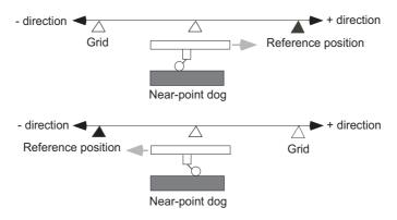
Axis without reference position Select whether the reference position is provided for the axis.
