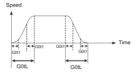
(Note) The time constant setting for the soft acceleration/deceleration can be changed by the setting of "#1219 aux03/bit7"
