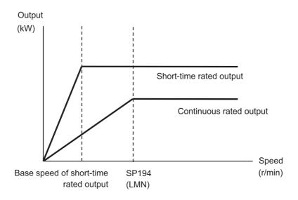
When "0" is set, the base speed of the short-time rated output will be applied.
