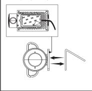
**4.** Clean the preferred location on the windscreen before installing the device.
