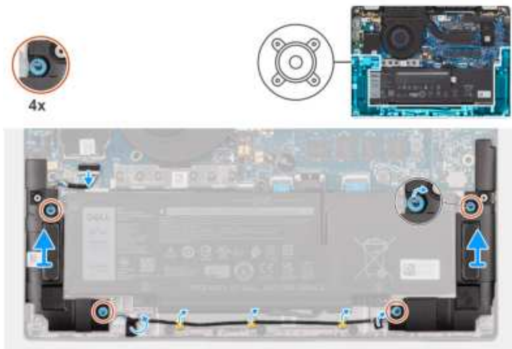
Figure 33. Removing the speakers for mainstream
