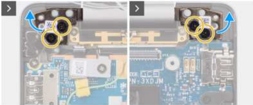
Figure 49. Removing the display assembly
