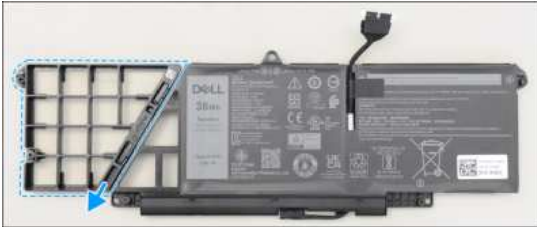
Figure 38. Removing the 2-cell battery
