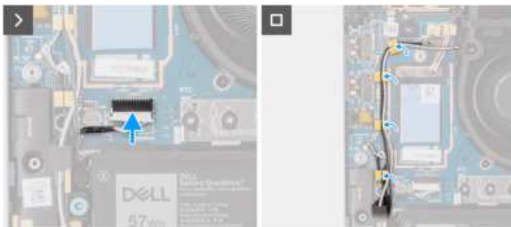
Figure 32. Installing the speakers for ultralight
