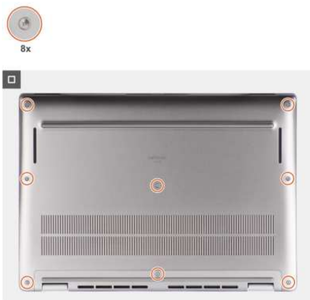
Figure 21. Installing the base cover
