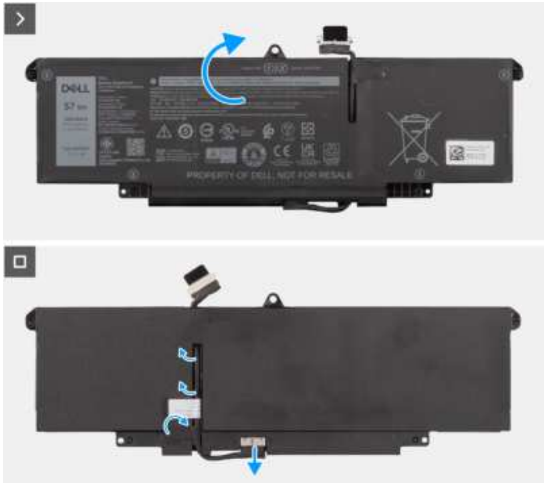
Figure 44. Removing the battery cable
