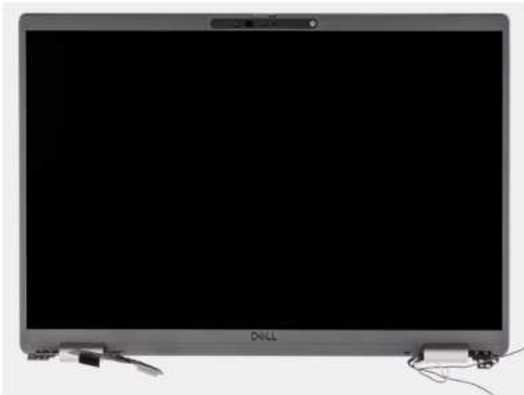
Figure 52. Display assembly with WWAN-antenna cables
