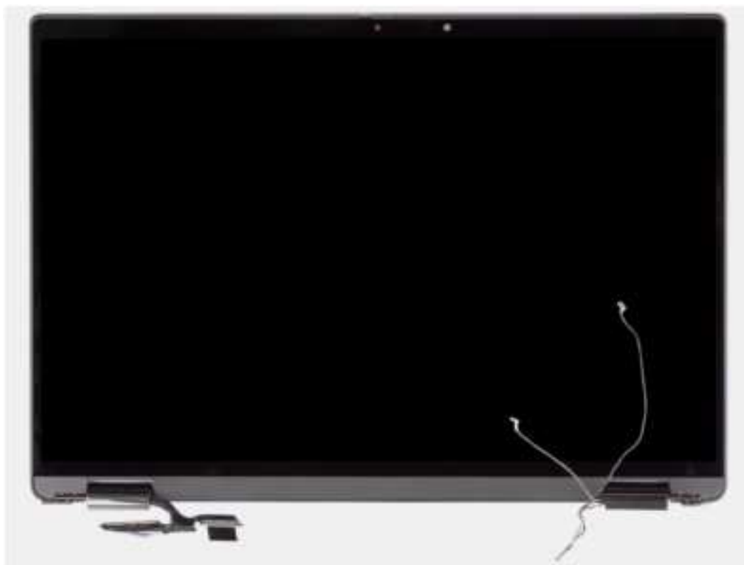
Figure 51. Display assembly with WWAN-antenna cables
