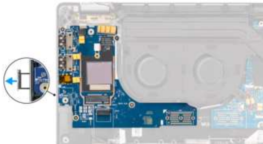
Figure 70. Removing the I/O daughterboard
