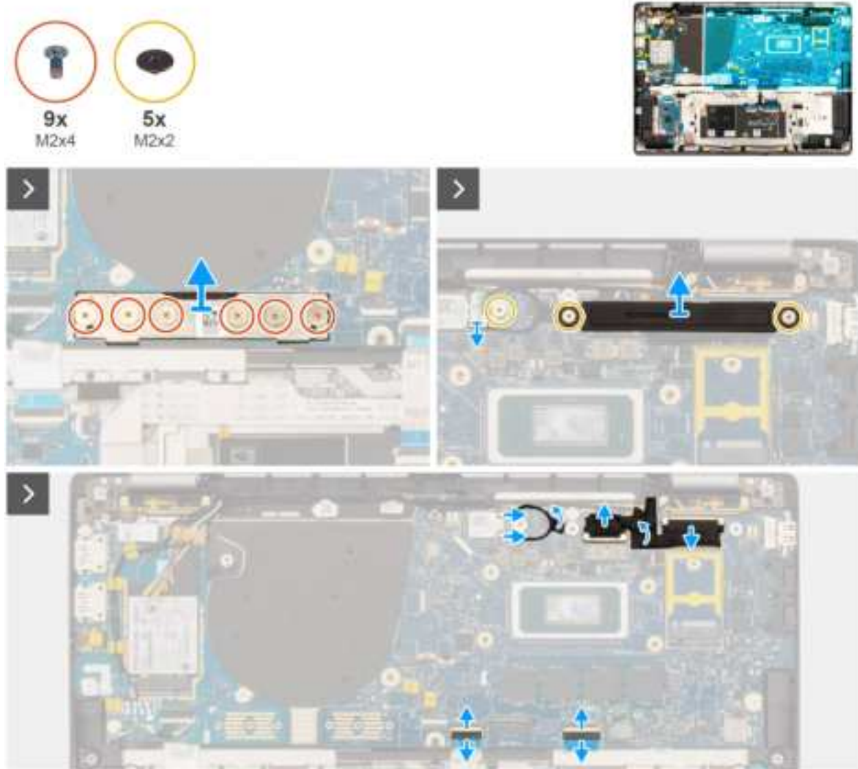
Figure 59. Removing the system board
