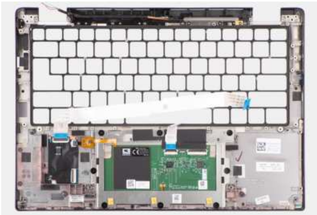
Figure 85. Installing the palm-rest assembly
