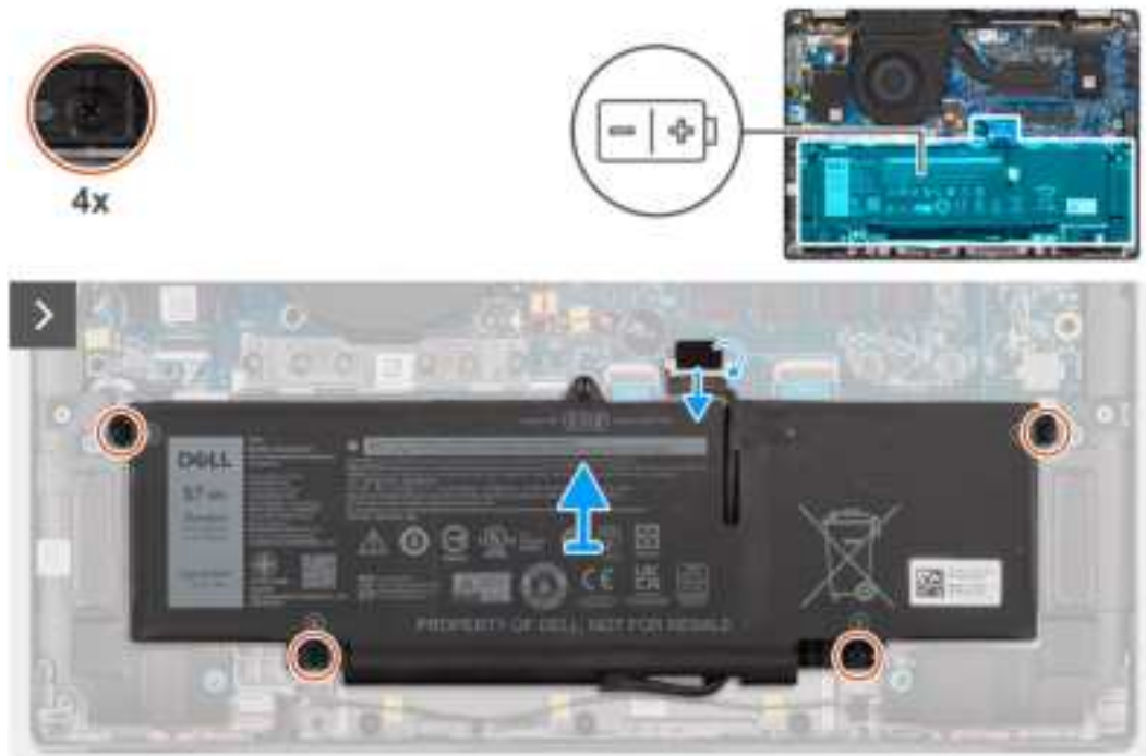
Figure 40. Removing the 3-cell battery
