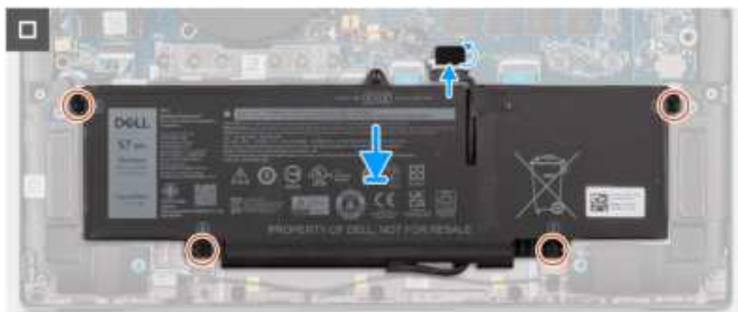
Figure 43. Installing the 3-cell battery
