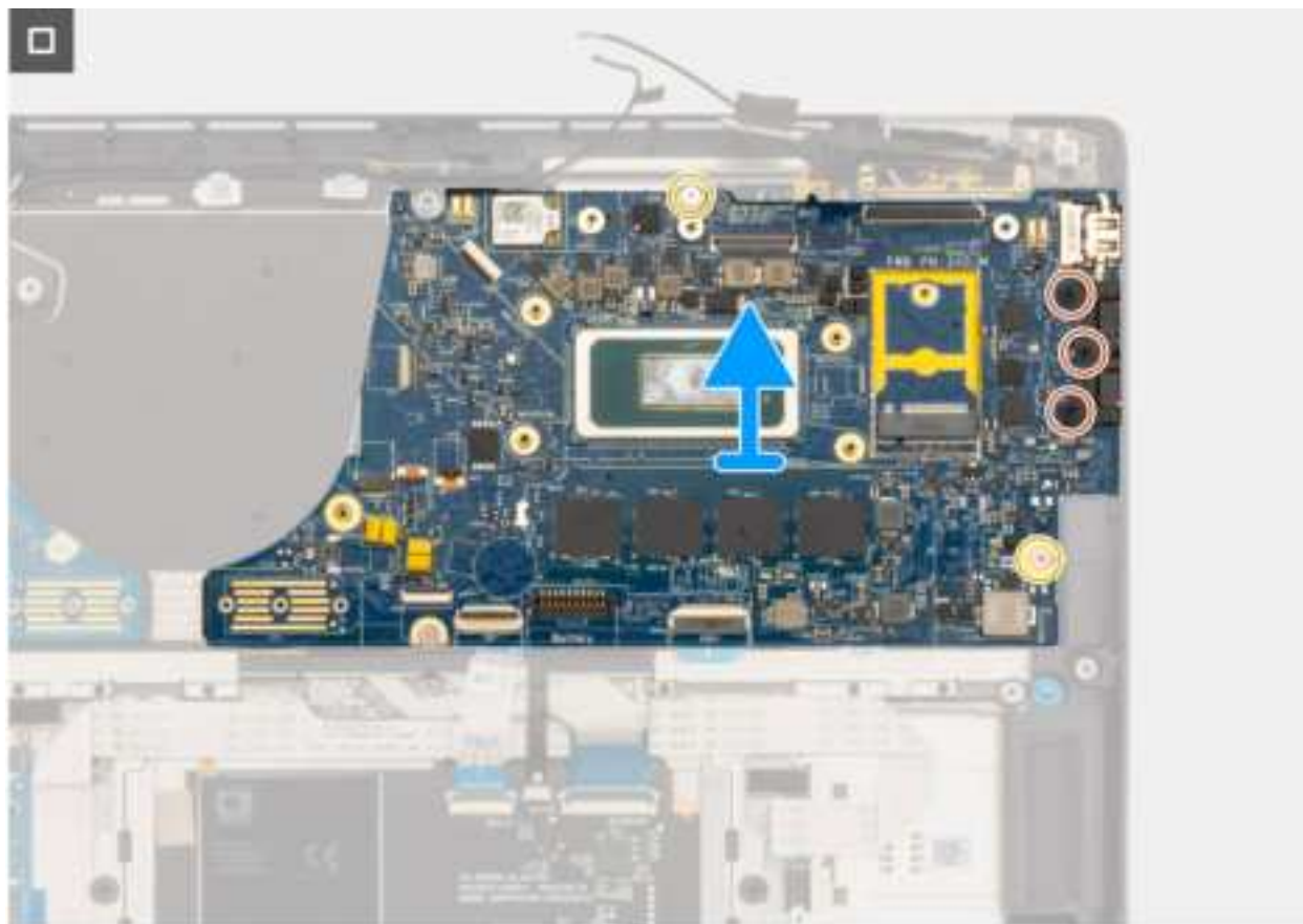
Figure 60. Removing the system board
