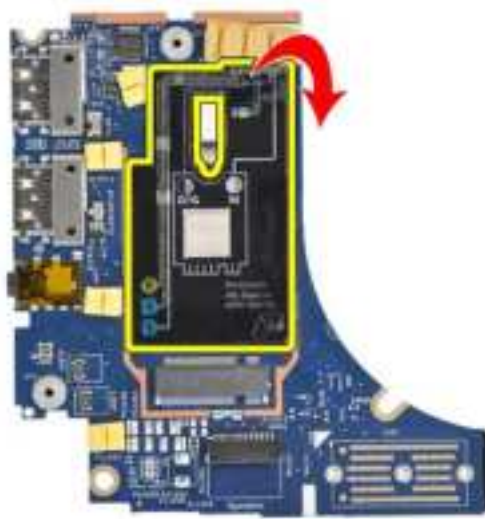
Figure 72. Latitude 7450 Clamshell 4G WWAN Configuration (Gasket Sticker)
