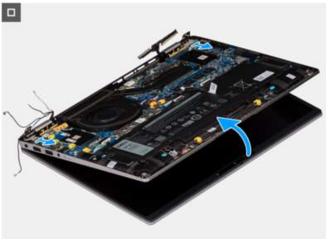
Figure 50. Removing the display assembly
