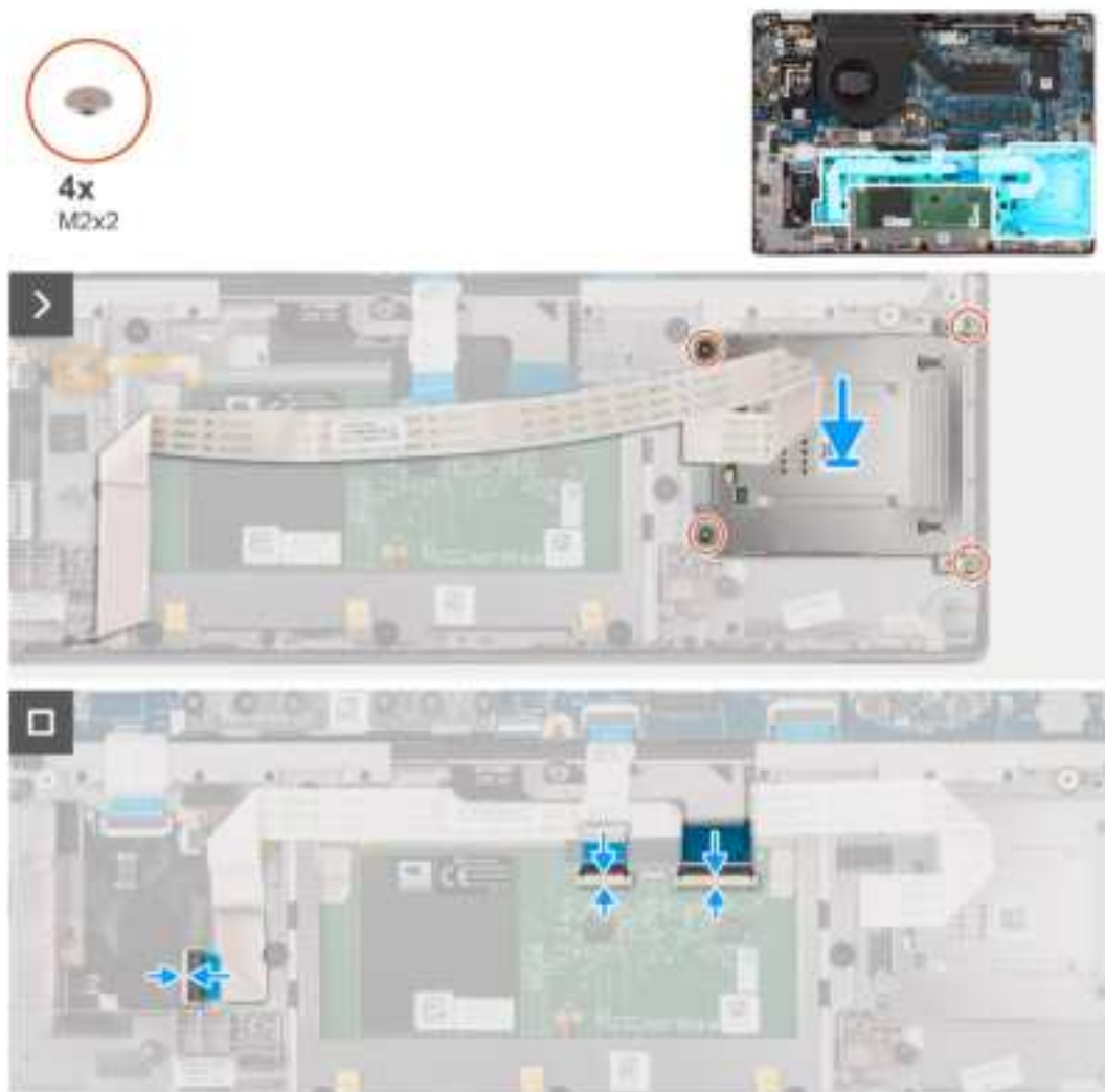
Figure 57. Installing the smart card reader
