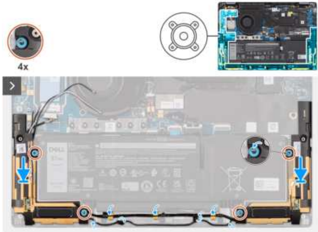
Figure 31. Installing the speakers for ultralight
