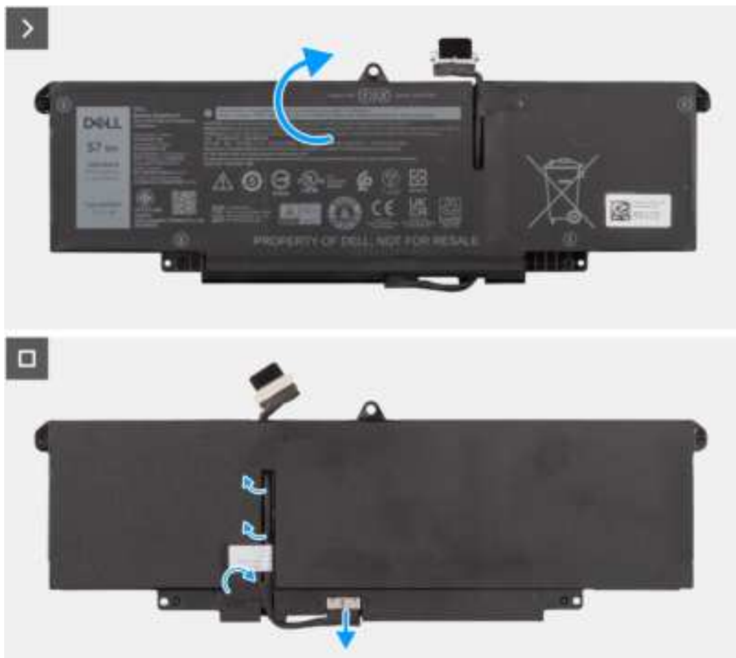
Figure 41. Removing the 3-cell battery
