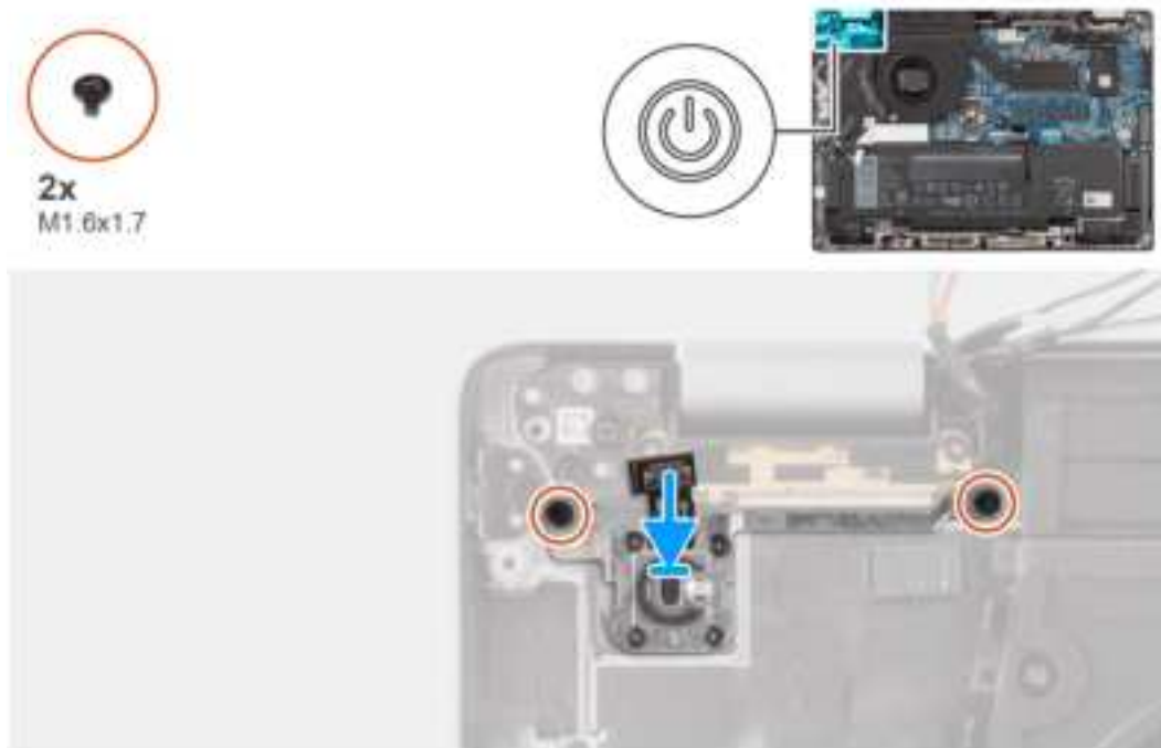
Figure 77. Installing the power button with optional fingerprint reader
