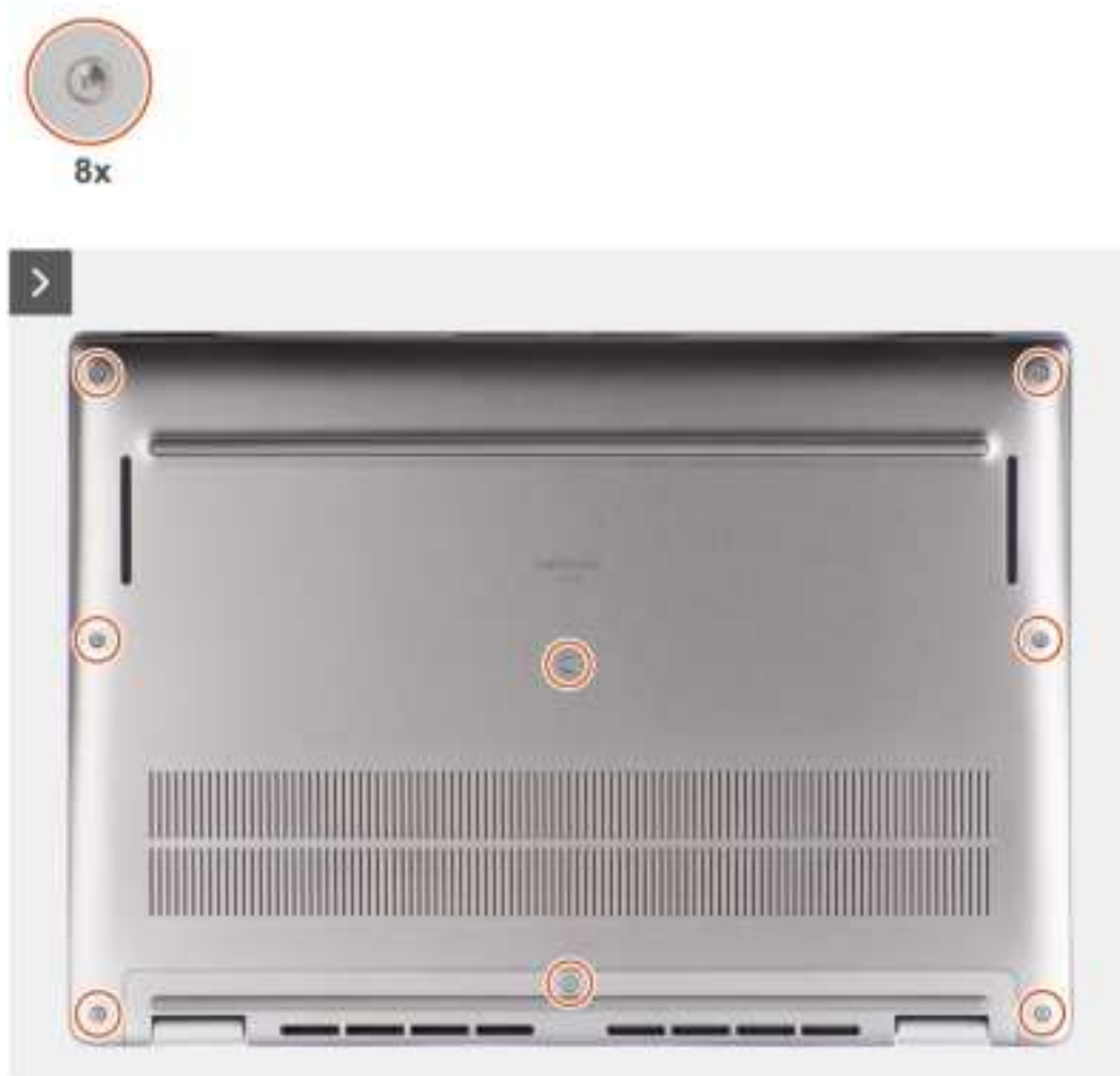
Figure 16. Removing the base cover
