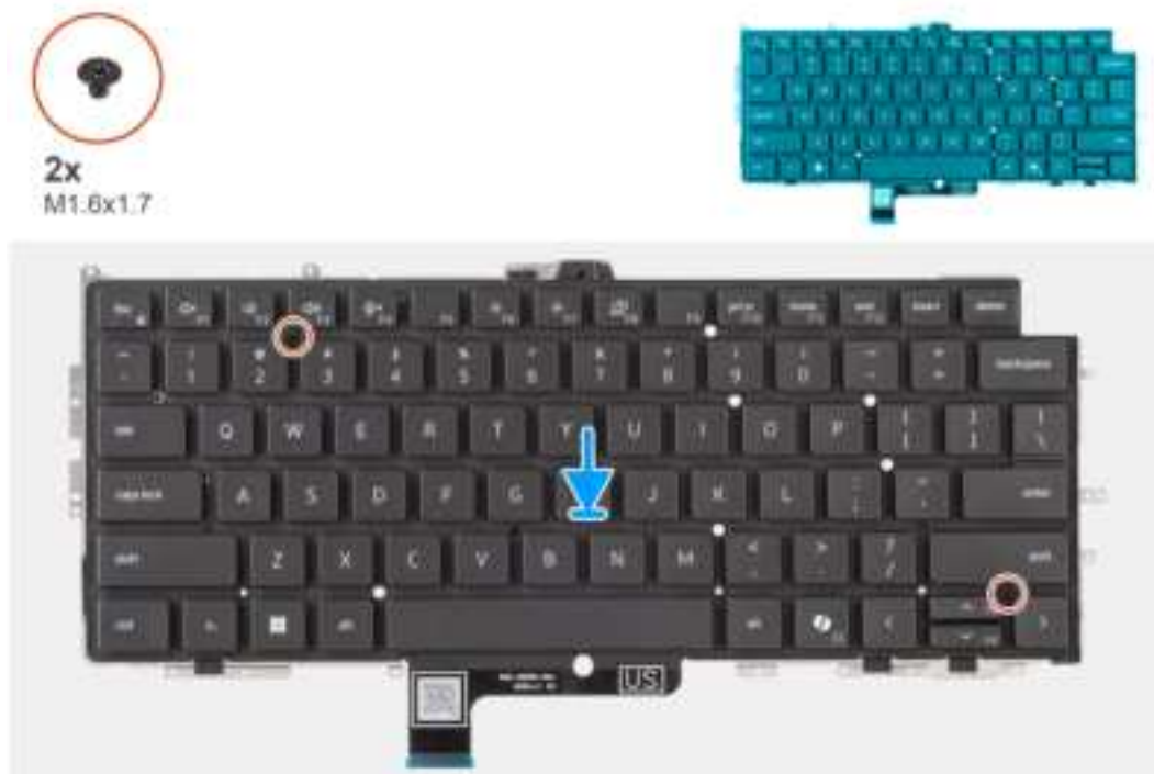
Figure 82. Installing the keyboard
