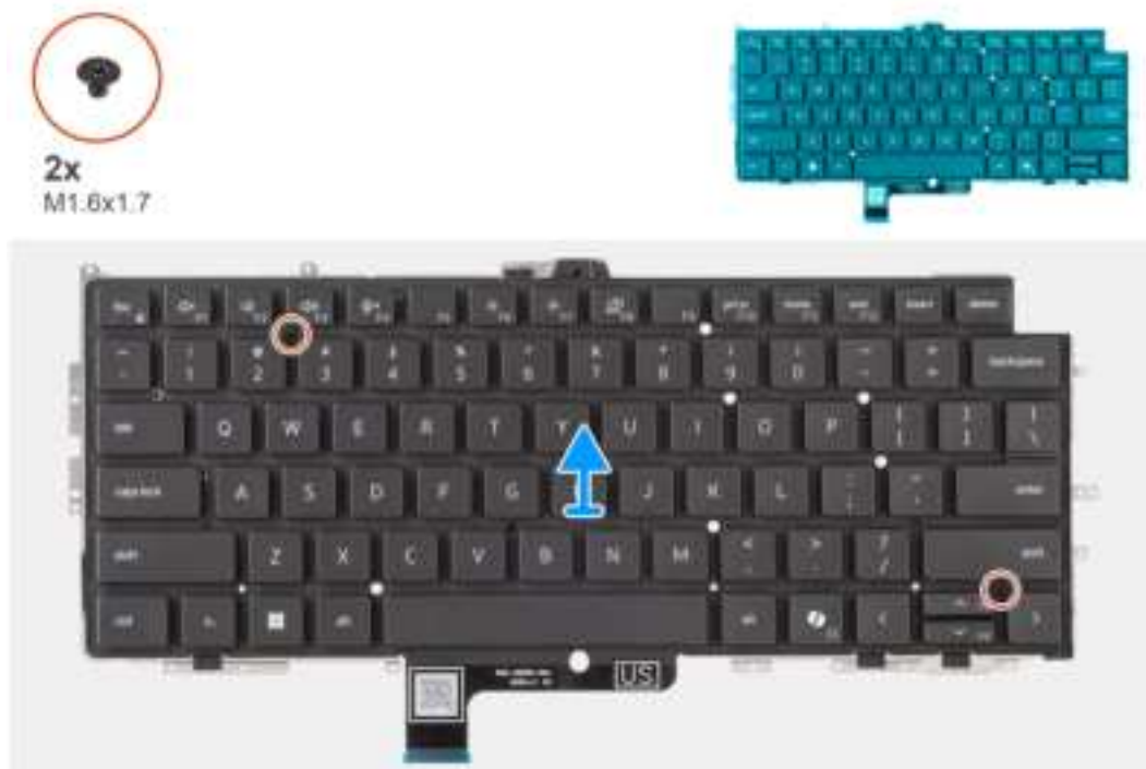
Figure 79. Removing the keyboard
