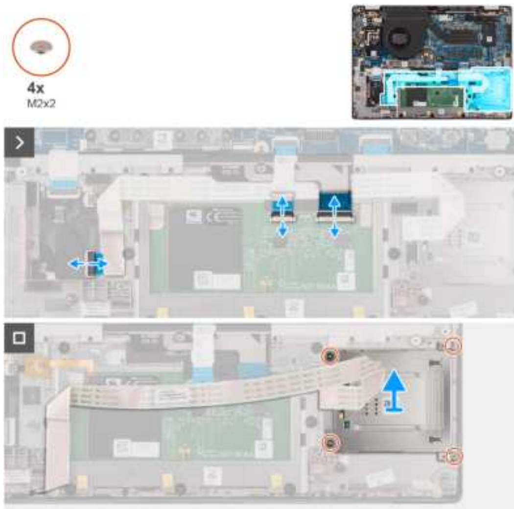
Figure 56. Removing the smart card reader
