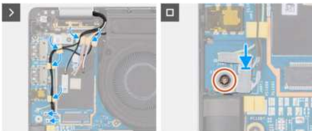
Figure 55. Installing the display assembly
