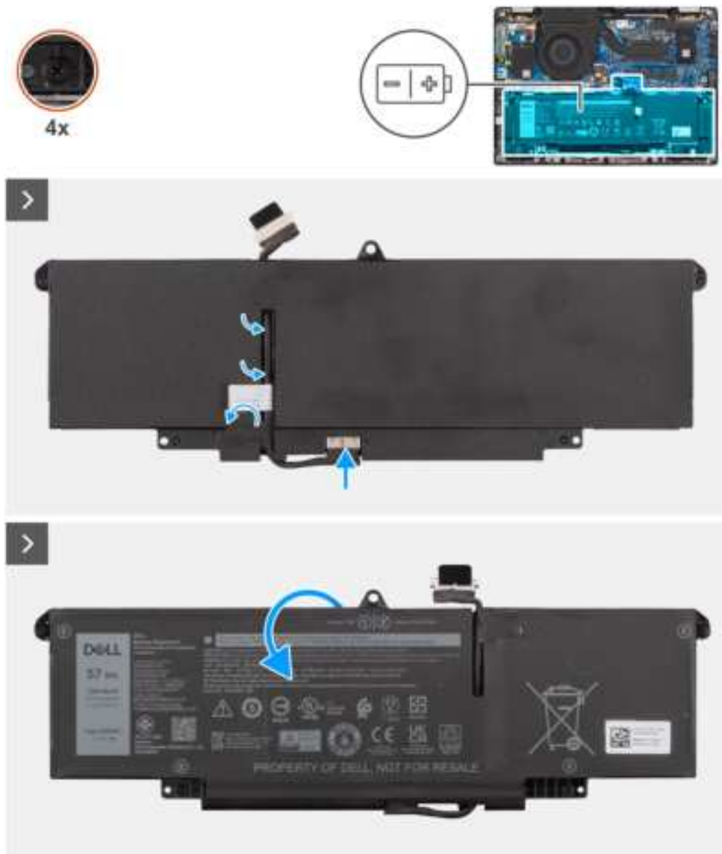
Figure 45. Installing the battery cable
