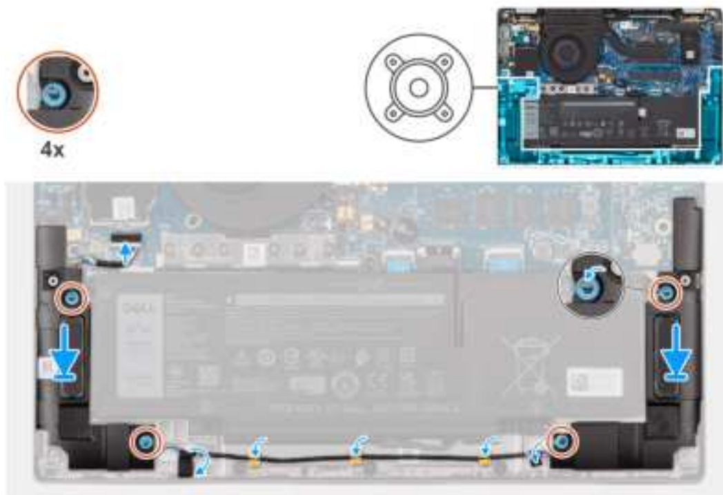
Figure 34. Installing the speakers for mainstream
