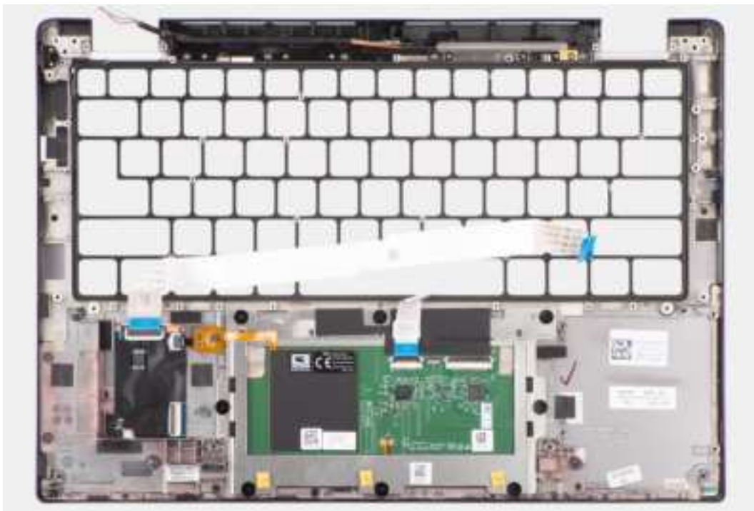
Figure 84. Removing the palm-rest assembly
