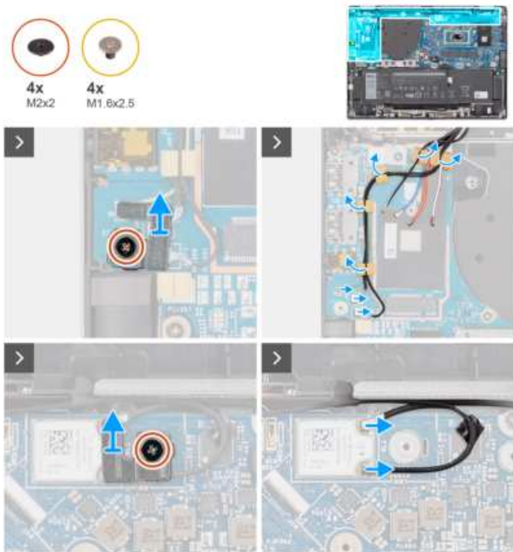
Figure 66. Removing the WLAN-antenna module
