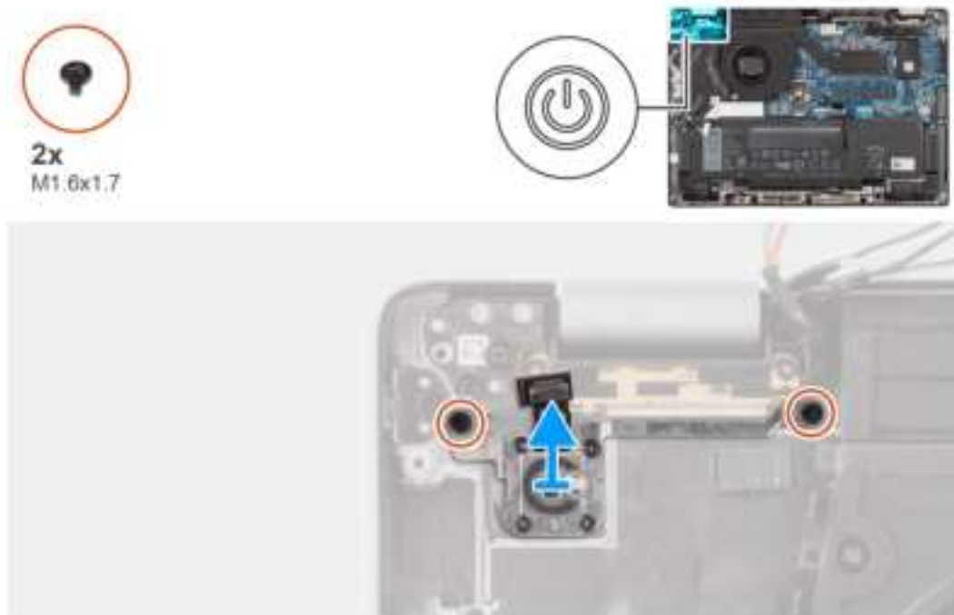
Figure 76. Removing the power button with optional fingerprint reader
