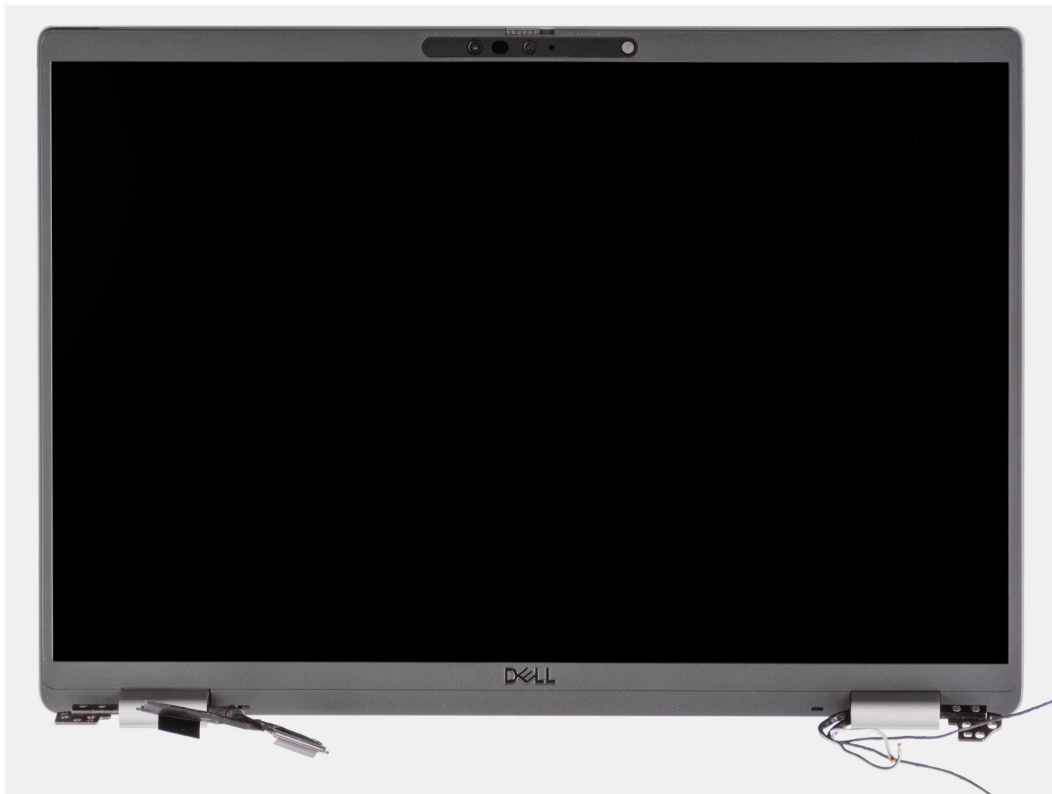
Figure 52. Display assembly with WWAN-antenna cables
