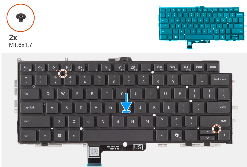
Figure 82. Installing the keyboard
