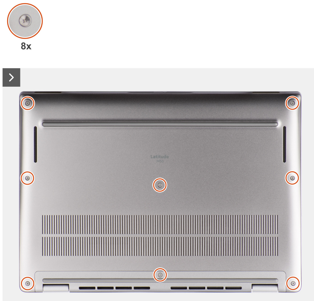
Figure 16. Removing the base cover
