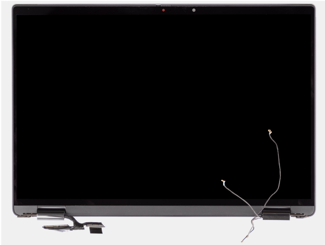
Figure 51. Display assembly with WWAN-antenna cables
