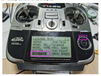
3. Map CH5 to the button, we map CH5 to SG stick in this example, you also can use other channel for mapping.
