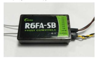
Connect PWM signal cable to corresponding receiver channel, GND to GND
