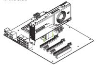
Install the graphics card into the primary x16 PCI slot. The Quadro RTX 8000, RTX 6000, and RTX 5000 are dual-slot GPUs and will cover the adjacent slot.
