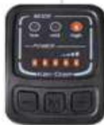
Press "+" again to move into pedal assist level "High". "High" is the maximum power of PAS.
