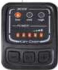
To switch on/off the E-Bike system, hold the
