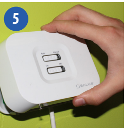
Clip the front of the unit back on by aligning the fittings and pushing into place.
