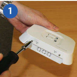
Loosen the screws at the bottom of the receiver unit.
