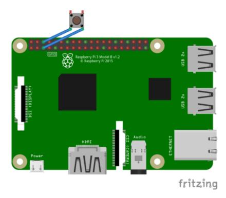
to connect the switch to the Raspberry Pi GPIO, plug a PIN on the GPIO3 (physical PIN 5 above on the left) and another on the mass located just to the right on the right (physical PIN 6):
