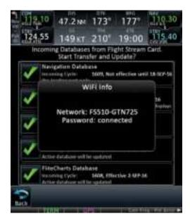
Flight Stream 510 Wi-Fi Network as Shown On GTN 750
