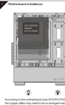
According to the motherboard type (ATX/M-ATX/ITX), the copper pillars may need to be re-arranged manually according to the fixing locations specific to your motherboard CPU Height limit: 175mm
