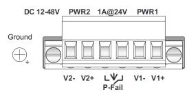
Wire Gauge: 12-24 AWG (3.31 - 0.205 mm2).
