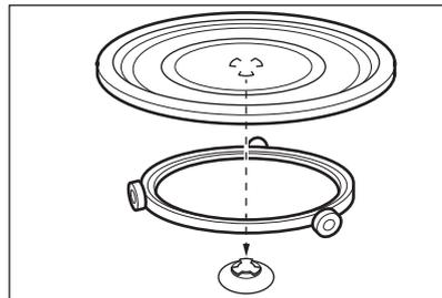
Use only the turntable set supplied with the appliance. Always cook food on the turntable set. Place the roller guide around the turntable shaft. Place the turntable glass on the roller guide. To allow the turntable set to operate properly, ensure that the indentations
