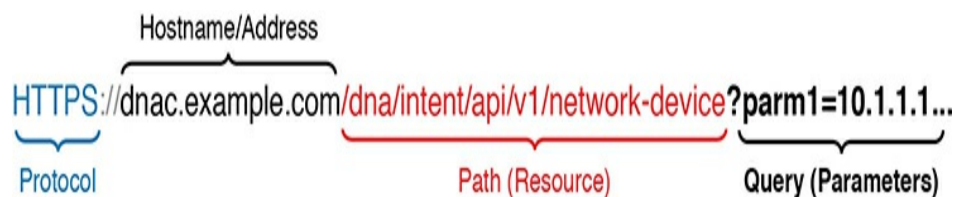
Figure 18-8 Example Components of a URI Used in a REST API Call
