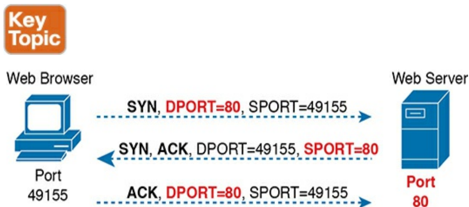
Figure 1-5 TCP Connection Establishment
