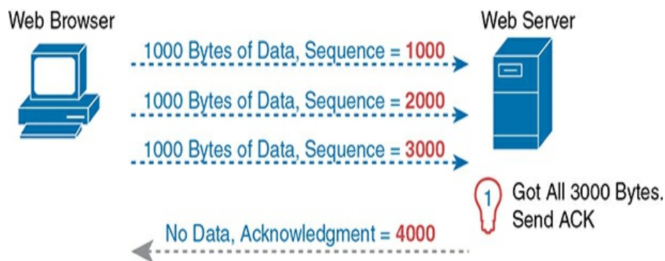
Figure 1-7 TCP Acknowledgment Without Errors
