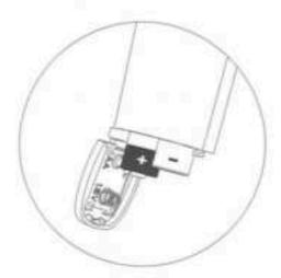
Once the batteries are installed and the battery cover is closed, press the Temperature Measuring button. The display will switch on and show:
