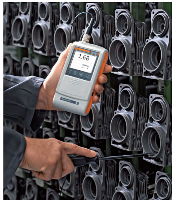
Measurements using the internal probe FAI 3.3-150
