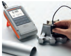
ISOSCOPE ® FMP30 using probe FTA3.3H
