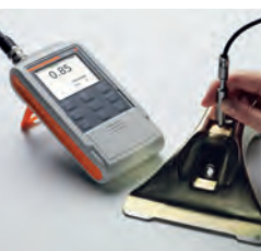
DELTA SCOPE® FMP10 using the probe FGAB1.3
