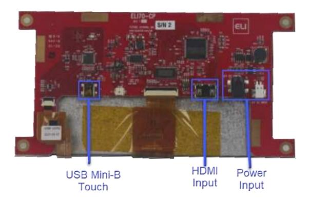
Power may be supplied either via the 2-pin terminal block J4 or via the 2.1mm power jack P2 (center positive)
