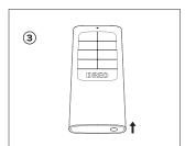
Push in the holder until securely locked into place.
