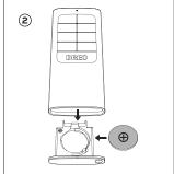
Replace the battery with the same type (CR2025 3V), making sure the (+) side facing up.
