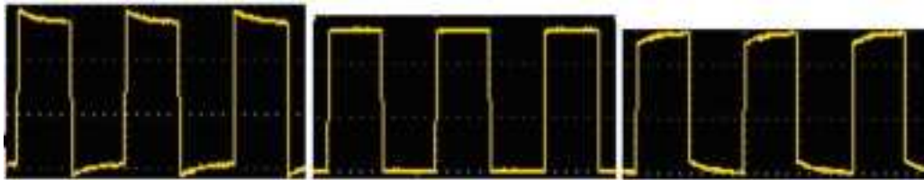
Overcompensated Compensated correctly Under compensated
