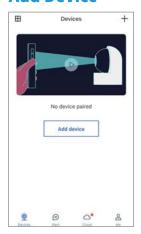
① Before adding a device on the APP, please be sure that your smartphone is connected to 2.4Ghz WiFi. 5Ghz WiFi is not supported.
