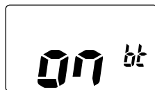
Battery voltage indication ON
