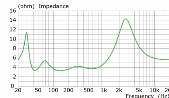
R3 Meta directivity contours - horizontal (top) and vertical (middle) - and impedance (bottom)
