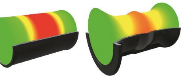
Figure 43. Pressure of the first resonance in a port with rigid walls (top) and flexible walls (bottom)
